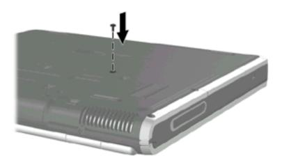
Replacing the hard drive retaining screw
